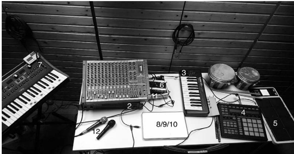
Abb. 1: Elektronisches Setup - 1 Mischpult: Behringer Eurorack MX 2642 2 Endstufe: t.amp E -800 3 Midi Keyboard: Alesis Q25 4 Sampler: Native Instruments Maschine Controller & Software 5 Drum Sampler: Roland SPD-30 Octapad, Roland KD-9 Kick Pad 6 Interface: Native Instruments Komplexe Audio 7 Analog Synthesizer: Moog Little Phatty 8 Laptop: Macbook Pro 13" 9 Software: Ableton Live 9 Suite 10 VST Plugins: Native Instruments Battery 4 / Rob Papen Predator 11 Mobiler Audiorecorder: Tascam DR-05 12 Mikrofone: Shure SM-58 / Behringer XM8500
